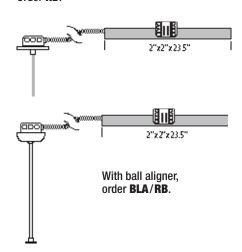
**NOTE**: Multiple drivers must be mounted no less than 4 inches apart side-by-side, and 1 inch apart end-to-end, to avoid overheating.
