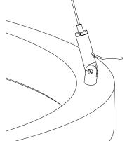
Insert cable ends into grippers, depress gripper nozzle to release/adjust cable. After final adjustments, leave approximately 1 inch excess cable.
