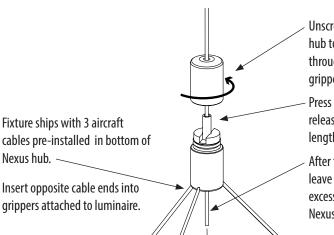
Unscrew Nexus cable hub top cap; insert cable through top cap and into gripper nozzle.
