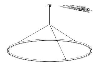
Remote driver housing has options for bar hangers for mount above suspended ceilings.
