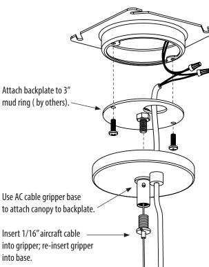
Make connections\* in J-box to remote driver. Connecting lamp cord to line voltage voids warranty.
