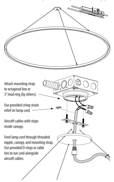
**NOTE**: Maximum canopy to fixture distance: 25 ft. Maximum canopy to driver distance: 100 ft. (with 10 AWG wire).
