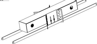
Polarity must be correct to ensure LED operation (connect wires red to red, blue to blue).
