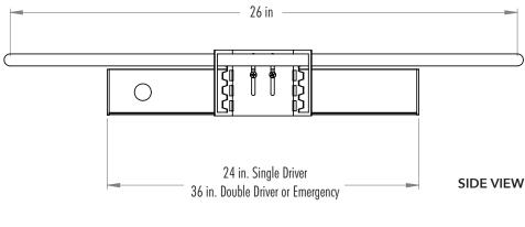
Remote driver housing has options for bar hangers for mount above suspended ceilings.
