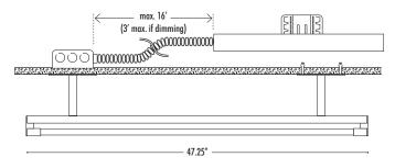
**NOTE:** Multiple drivers must be mounted no less than 4 in. apart side-by-side, and 1 in. apart end-to-end, to avoid overheating.
