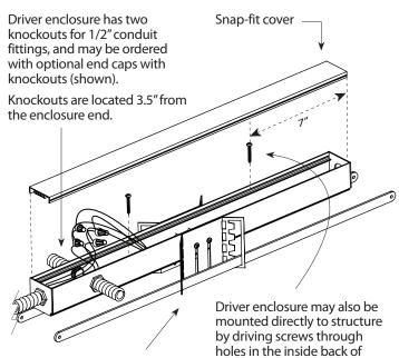
Bar hangers (included) may be used for suspended ceiling mount (or removed if not needed).
