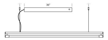
**NOTE**: Drivers must be accessible after installation, and must be mounted no less than 4 inches apart side-by-side and 1 inch apart end-to-end, to avoid overheating.
