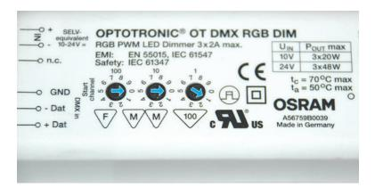
For proper operation, confirm that the interface PWM dials remain on the factory preset of channel 1 (001), on all control interfaces, in all fixture driver housings connected to the Traxon controller.
