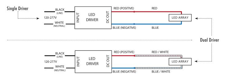
NOTE: Load is split between two drivers, the lamp cord four conductors; red, black, white, and green.
