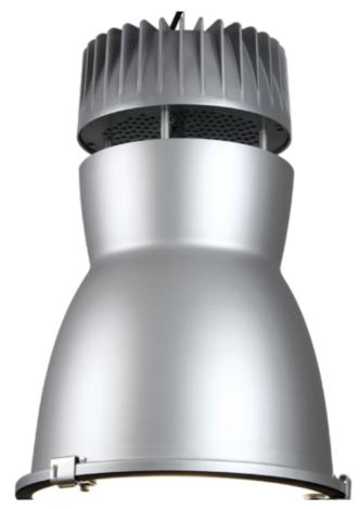
Mminimalist redesign of classic industrial high bay fixtures, with finned driver housing, anodized aluminum reflector, and tempered soda lime glass lens. 13 in. diameter aperture.
