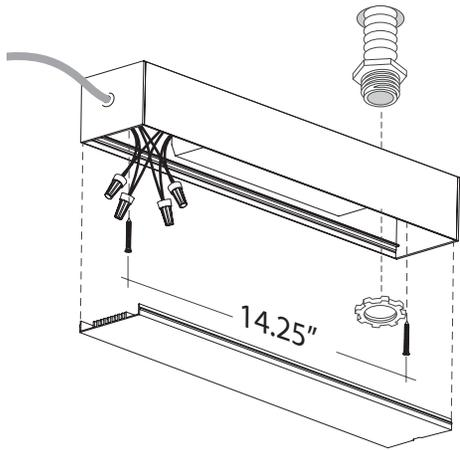
Mount drive housing to surface with screws.
