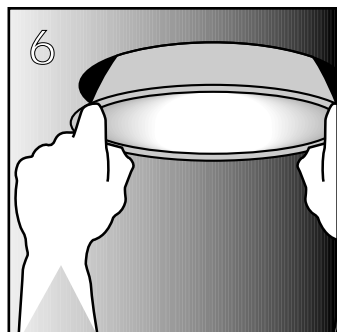
Slide reflector into frame, insert proper lamp and check operation
