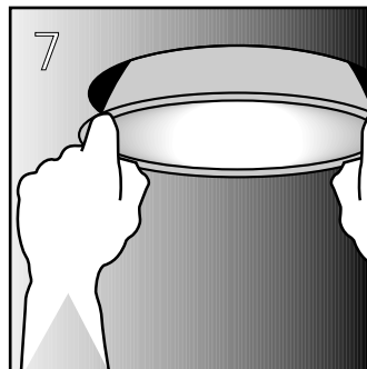
7 Slide reflector into frame, insert proper lamp and check operation
